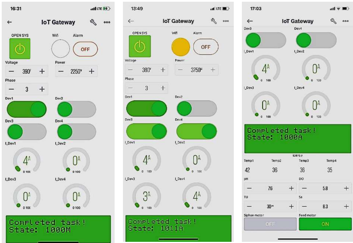
Figure 10. A capture of the smartphone control app for the MFC. From left to right, a capture of MANUAL mode, AUTO mode and the lower part of the app page.
