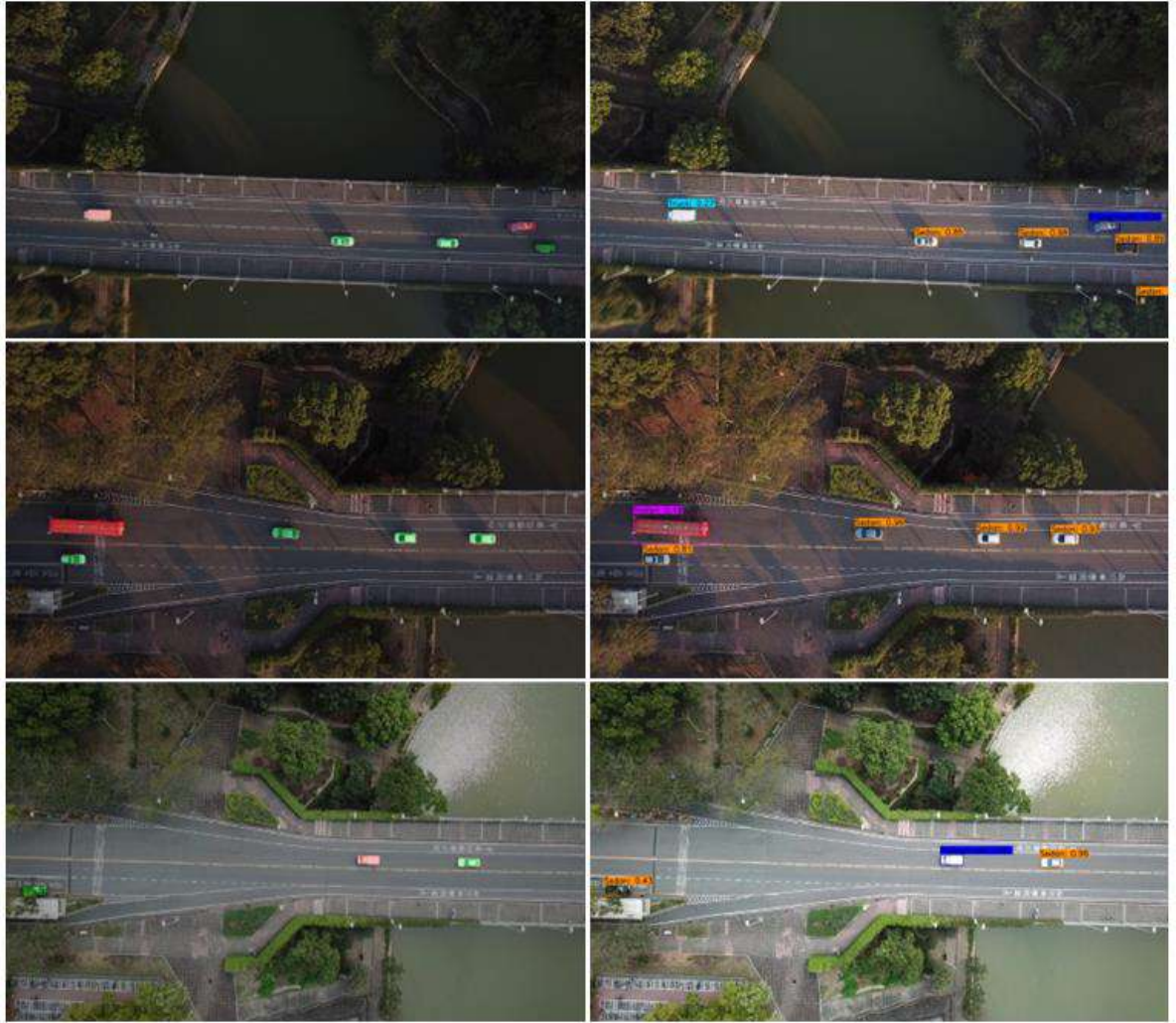
Figure 3: Our experimental results from our dataset, the left images are our semantic vehicle segmentation, and the right image is our vehicle detection based on YOLOv4.
