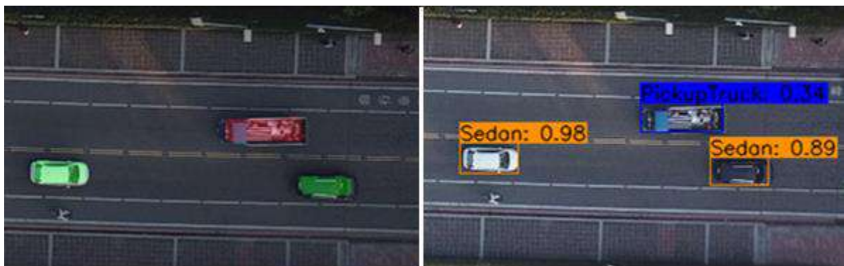
Figure 1: Overview of our vehicle classification on aerial images, the left image is semantic vehicle segmentation, and the right image is vehicle detection on YOLOv4.
