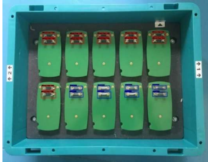
Figure 5. Our experimental results were tested on a stored box with many circuit boards. Red and blue colors are without a fuse and with a fuse on the circuit board, respectively.
